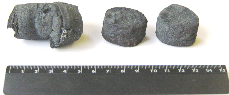
Fig. 2. Appearance of the samples obtained by thermal synthesis from the mixture powders of titanium hydride, aluminum and carbon
